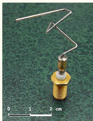
Figure 7: NASA’s ST5 satellite antenna, designed via evolutionary algorithms to meet the stringent and very specific requirements of the mission. It is the first such object to have been sent to space (2006).
